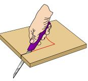
Use the broken fire brick component as a template and easily cut out a section of Fire Tech to make a replacement.
