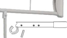
Note that in relation to the version with the support leg; a simple to adjust clip is fitted which enables three variations in the length of the leg to be chosen.
